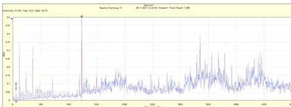
Fig. 8. Spectrum of vibration of differential gear at the 5th speed degree [4]
