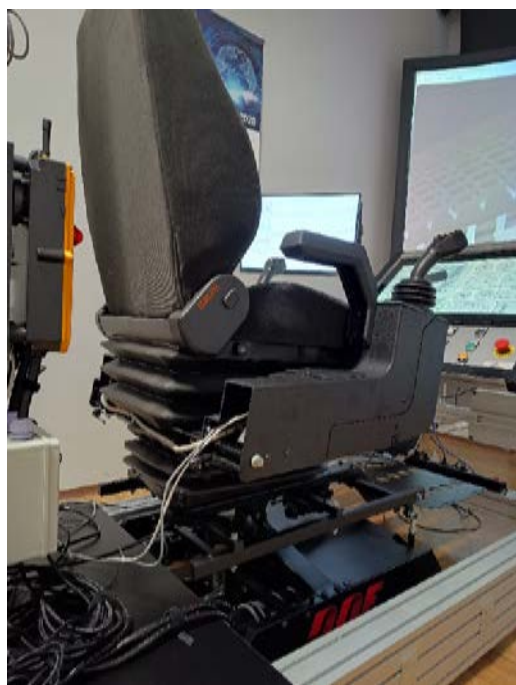
Fig.1 DOF Reality HERO H3 platform built into the base of the {RH-Sim} roadheader simulator (a-c) and control device (d)
